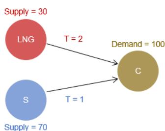
In order to make the above arguments concrete, consider the simple network depicted on the left, constituted by one supplier  $S$ , one LNG node and one consumer node  $C$ .
