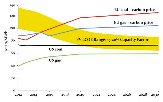
Figure A3: Levelised cost of electricity from PV, coal and gas - 2012-2030
