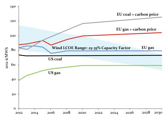
Figure A4: Levelised cost of electricity from wind, coal and gas: 2012-2030
