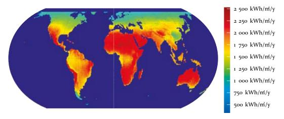
Figure 4: The solar flux at the earth's surface over the year
